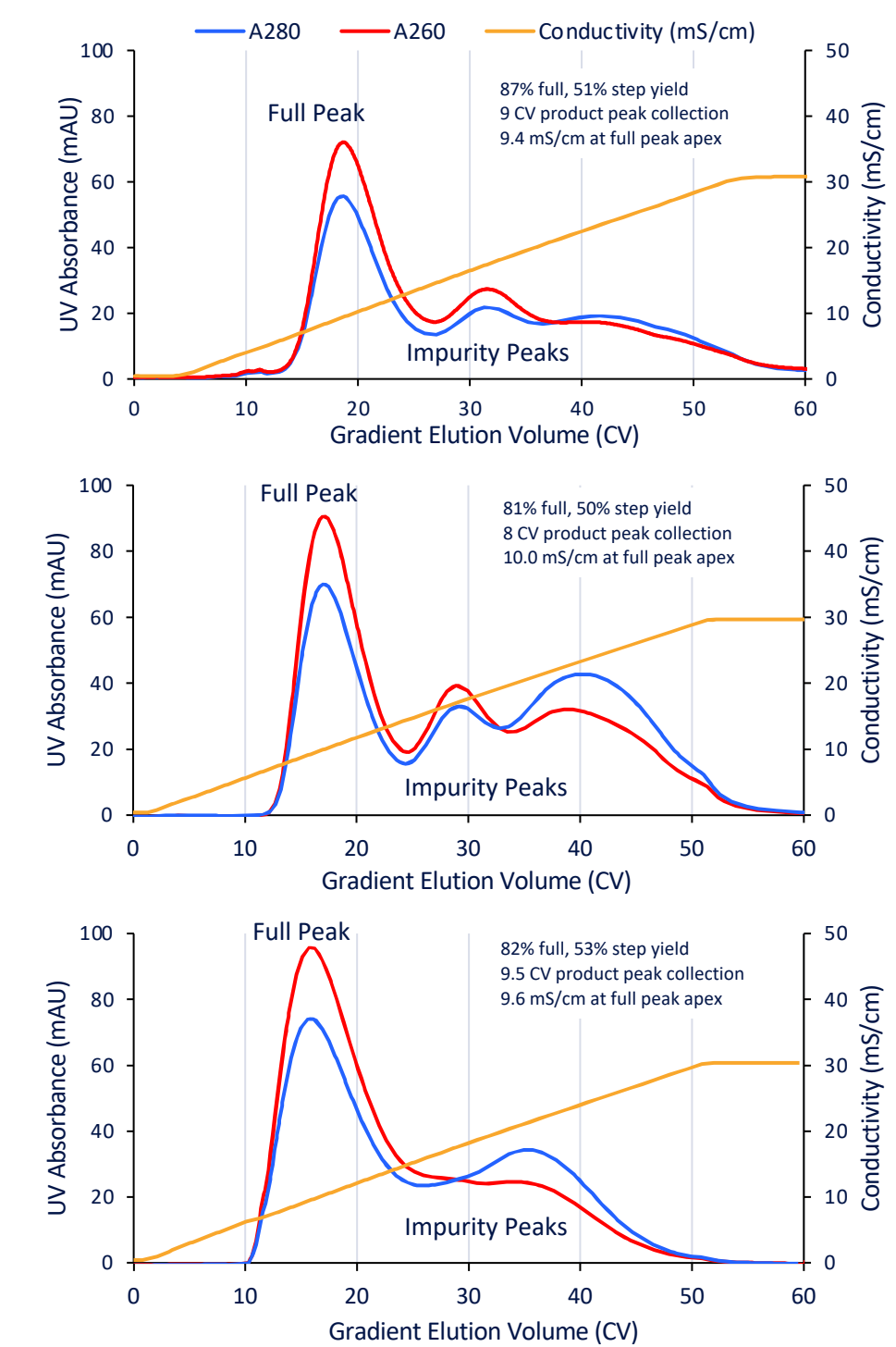
Figure 1. Example Gradient Elution Chromatograms Performed with Different Batches, Scales, & Laboratories
